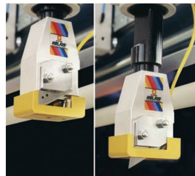
fig. A: NOT IN WORK fig. B: IN WORK
