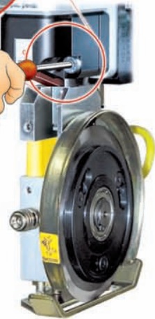
Fig. 3: Screw unlocking for cutting angle adjustment
