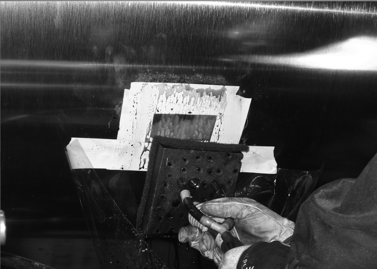
Brushplating of dryer
