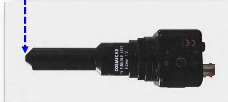
Inside housing pinhole lens and GigE camera
