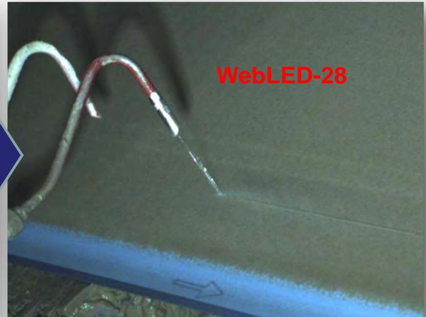
**Existing lighting** – analog colour camera with poor quality light – shutter 1/500<sup>th</sup> sec
